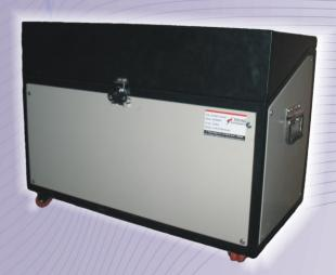
In all Power and Distribution Transformers, Switchgears and Circuit Breakers etc., transformer Oil or other insulant is a very important ingredient. Used liquid insulant should have a very high dielectric strength. To test the dielectric strength of the insulant, a very high voltage is passed through it. The failure of the dielectric strength of insulant is shown by a spark across two electrodes.
